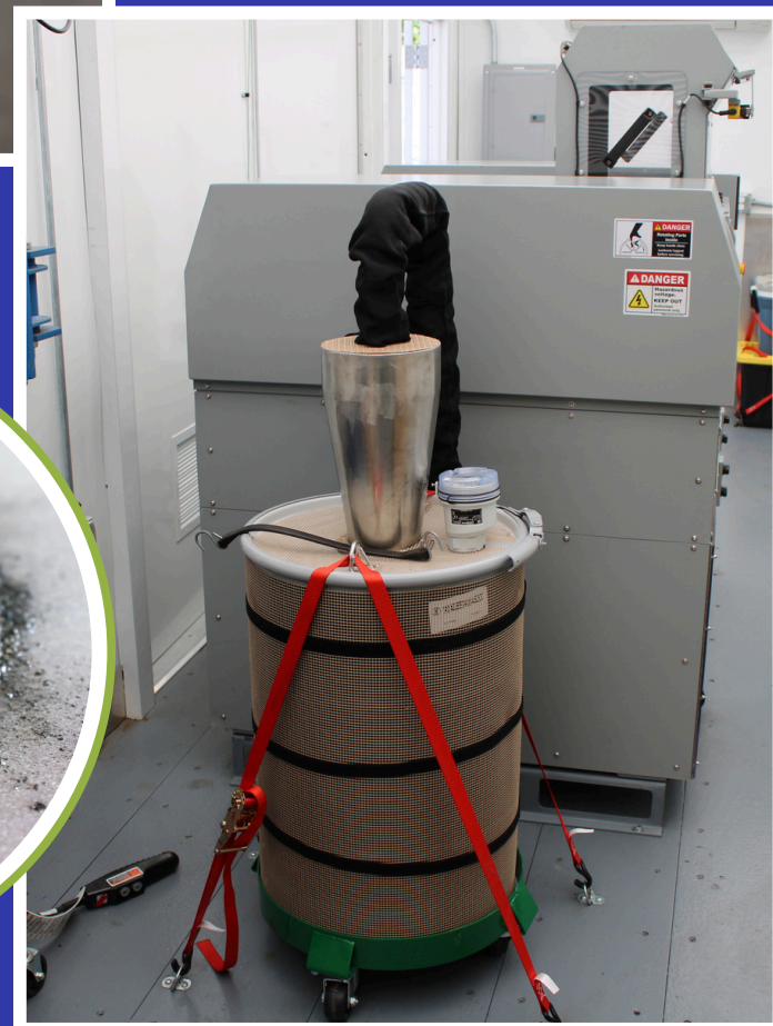
30-Gallon Debris Collection: Equipped with level sensing for efficient operation.
